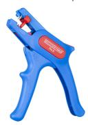
The WEICON Wire Stripper No. 5 has an adjustable length stop from 5 - 12 mm. This allows all flexible and solid conductors of 0.2 –  $6.0\ mm^2$  (24 – 10 AWG) to be stripped. The length stop can be removed if required. An easy-to-access side cutter is integrated into the tool and can be used up to a cable diameter of 2 mm. It also has exchangeable blades.
